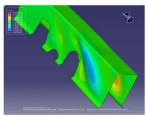
Figure 2: Transverse Frame Shear Web Skin Wrinkling
