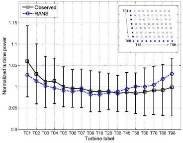
Comparison of CFD and measured data for the perimeter turbines at Horns Rev 1 (Bleeg et al , 2018)
