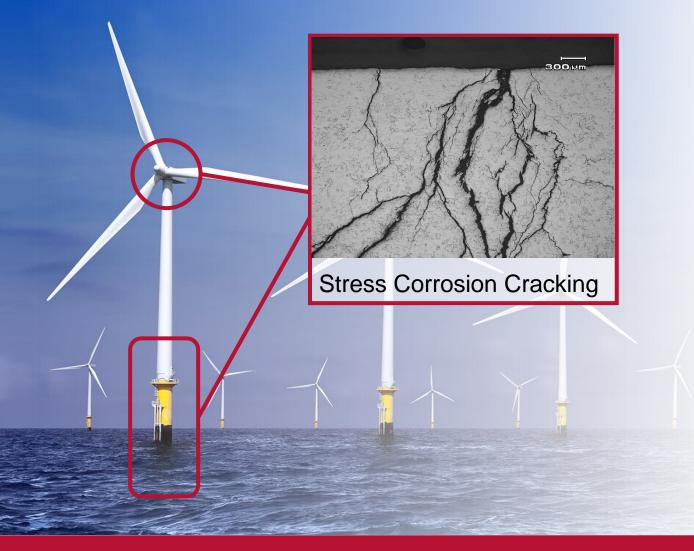
Material susceptible to SCC SCC Tensile Stress
